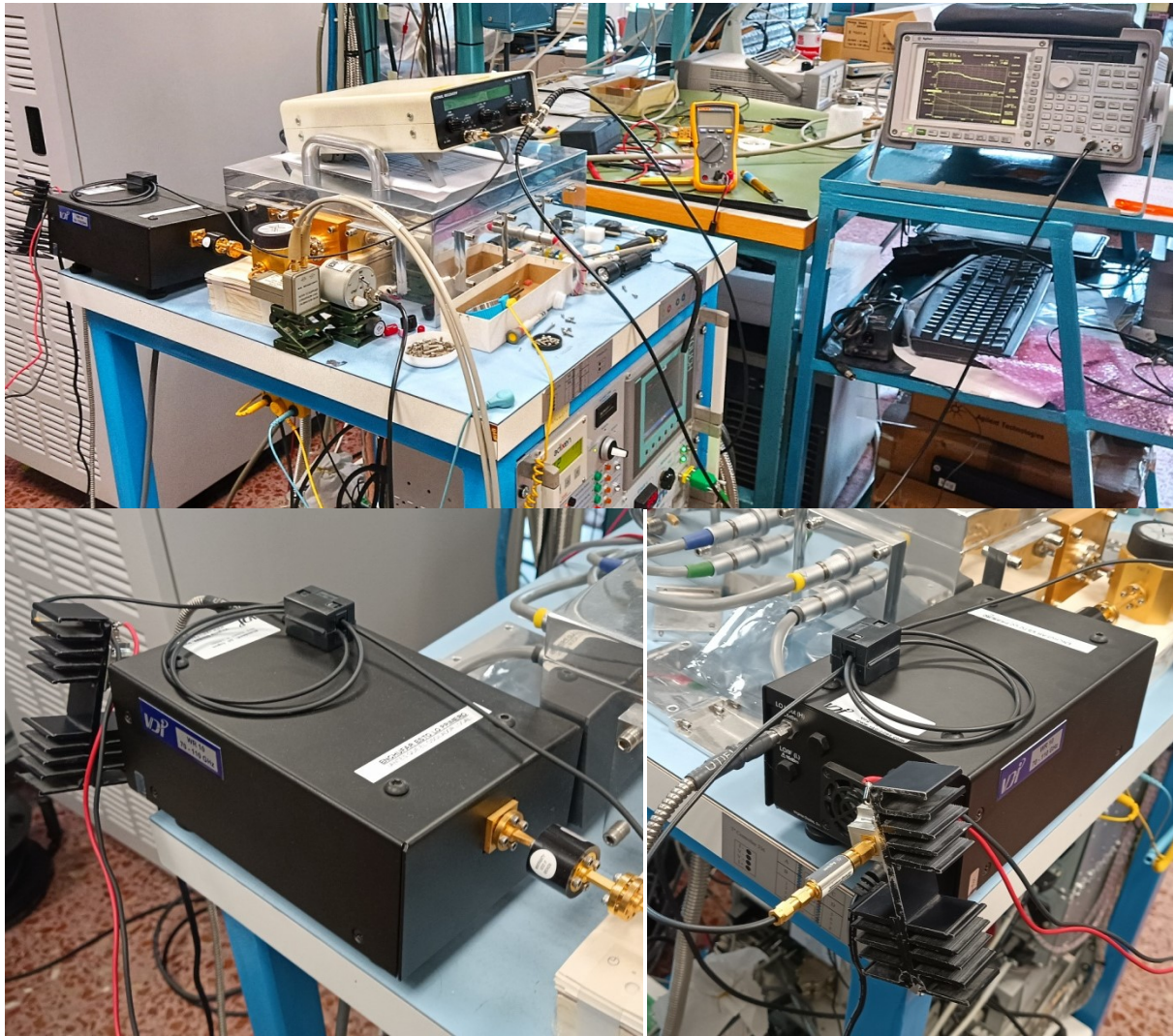
Figure 2: Up: Test setup used for the measurements. Down: Details of the Virginia Diodes Converter with isolator at the input and MITEQ amplifier and detector connected directly at the output.
