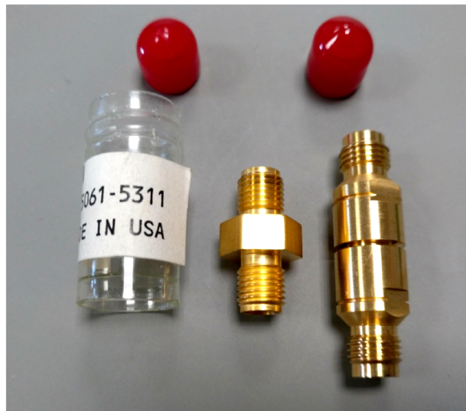
Figure 1: Photo of the transitions used to connect the power sensor to the port 1 of the PNA-X for power calibration. Left: a short 3.5 mm female to female PN 5061-5311 used for measurements up to 26.5 GHz. Right: metrology grade 1.85 mm female to female PN 85058-60114 (included with N4694A E-cal module)
