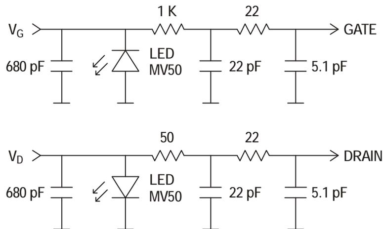
**Figure 3:** YCF 4 bias circuits (inside the amplifier)
