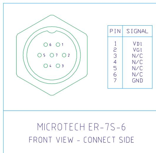
**Figure 1:** DC Connector pinout
